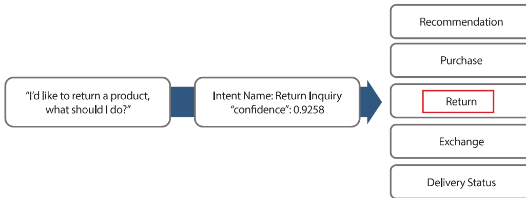
Figure 4. Matching a natural language question with prepared menu in robotic process automation.
